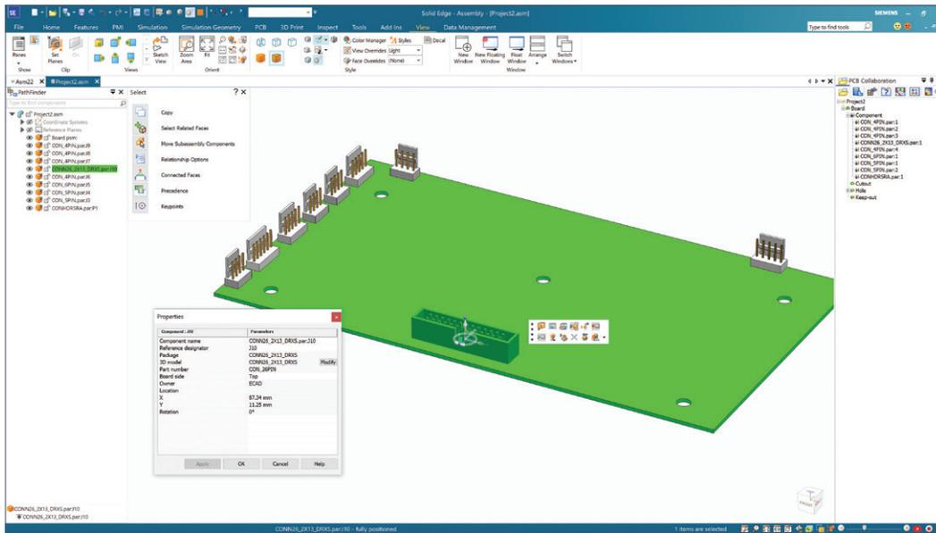
allowing users to select data for import and export on a need-to-know basis. Older formats, such as the intermediate data format (IDF), overload communication by transferring more design data than is necessary. By transmitting only relevant data for change proposals, intellectual property is preserved. This is particularly important when the design is spread across different companies. Solid Edge PCB Collaboration supports IDX 2.0 and 3.0.
