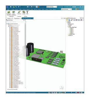
with MCAD users able to initiate PCB design from within Solid Edge. Design aspects are sent between ECAD and MCAD until clearances and electromechanical interferences are checked and all modifications are made. This process continues until all parties are satisfied with the design.
