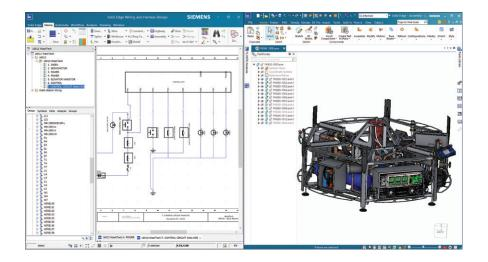
solution provides interactive, highlighted cross-probing and updating between the ECAD and MCAD domains.
